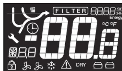
Subsequently, the selected program will be shown on the secondary display - "P05" in this case. The program "P05" controls 2 compressors. Hence both compressor symbols will light up in blue.
